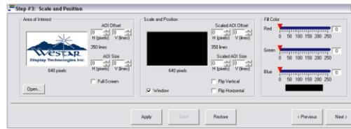
The areas of interest within the input image and the mapping to the output resolution, thereby defining windowing and scaling functions
